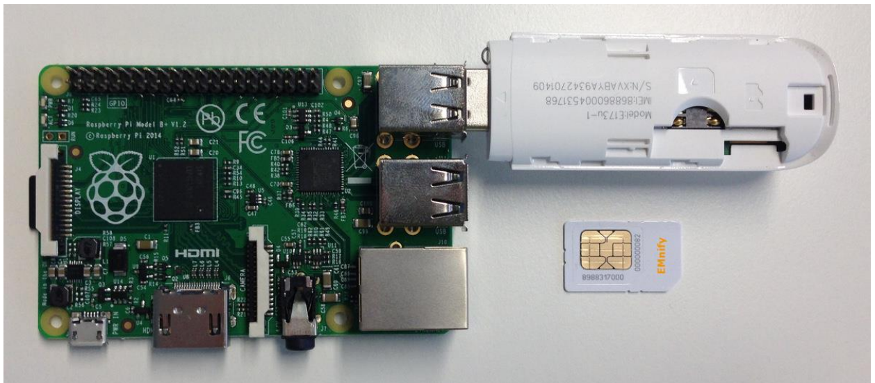
Figure 11. Raspberry Pi 3 Model B with a Huawei LTE USB Modem (Permission Pending) [62]
